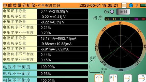
Unbalance - 3-phase 4-wire test interface
